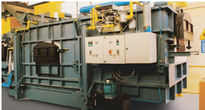
Air/gas ratio control on melting furnace for ensuring stoichiometric combustion over the entire capacity range
